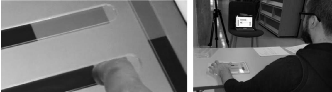
Figure 5. Eyes-free use of the touchscreen enhanced by the addition of a Perspex guiding layer
