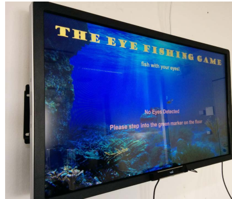
Figure 1: The Eye Fishing game deployed on a 42 inch public display equipped with a Tobii REX. The idle page guides the passersby to step into a green marker on the floor to be in range of the eye tracker and start interacting.
