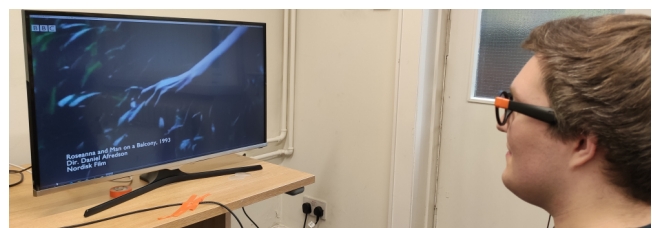
Figure 1: A TV viewer wears a pair of acoustically transparent Bose Frames, hearing the intermixing of both TV and Frames audio (shown lit, lighting was dimmed for study).
